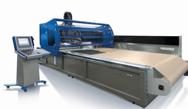
Moving enclosure and automatic feed
