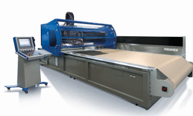
Moving enclosure and automatic feed
